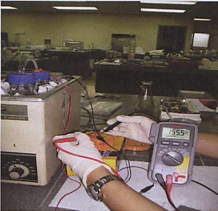
Figure 13 MFCs demonstrating power generation from microbes utilizing laboratory broth as the biofuel
