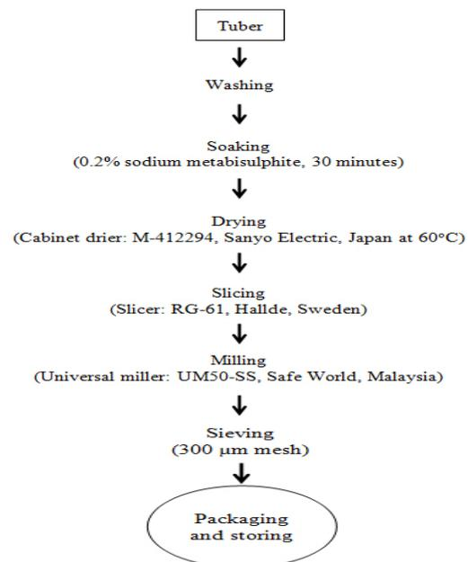
Figure 1. Flow diagram of sweet potato flour processing
