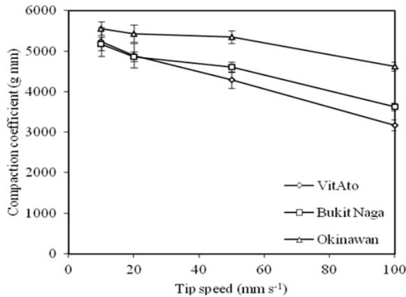
Figure 5. Compaction coefficients of sweet potato flours
