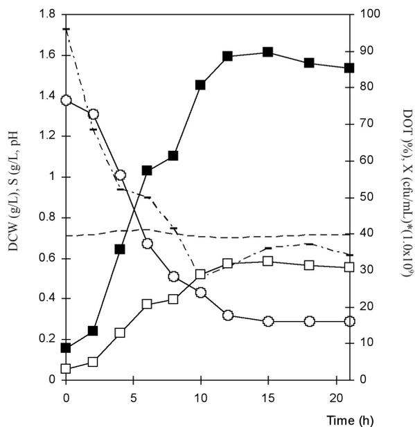
Fig. 1: The time course of batch fermentation using glycerol as the carbon source in a 2 l stirred tank fermenter. Symbols represent (◆) cell count,  $X$  ( $\text{cfu ml}^{-1} \times 10^9$ ); (.....) dissolved oxygen tension, DOT (%); (◇) pH/10; (■) dry cell weight, DCW ( $\text{g l}^{-1}$ ); (○) glycerol concentration,  $S$  ( $\text{g l}^{-1}$ )
