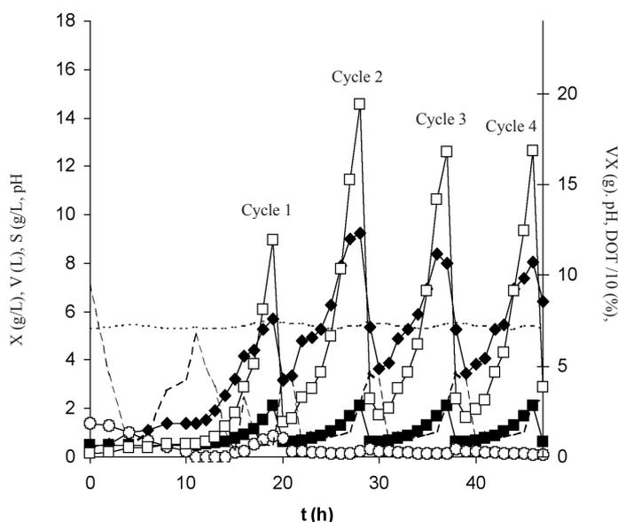
Fig. 4: Repeated exponential fed-batch culture of *Bacillus sp* operated at  $\mu = 0.4 \text{ h}^{-1}$ . Symbols represent ( $\blacklozenge$ )  $X$ ; ( $O$ )  $S$ ; ( $\blacksquare$ )  $V$ ; ( $\square$ )  $VX$ ; (---)  $pH$ ; (—)  $\%DOT/10$ . Arrow indicates the start of feeding for the fed-batch fermentation at each new cycle
