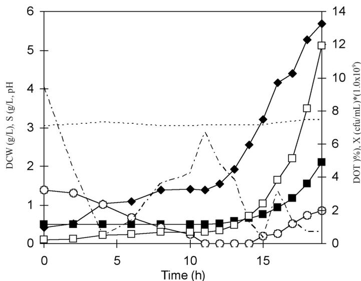
Fig. 3: The time course of the exponential fed-batch fermentation at  $\mu = 0.40 \text{ h}^{-1}$  using glycerol as the carbon source in a 2 l stirred tank fermenter: Airflow was increased to  $4 \text{ L min}^{-1}$  at 900 rpm after 17 h. Symbols represent (◆) DCW; (○) S; (■) V; (□) VX; (----) pH; (\_\_\_) % DOT/10. Arrow indicates the start of feeding for the fed-batch fermentation
