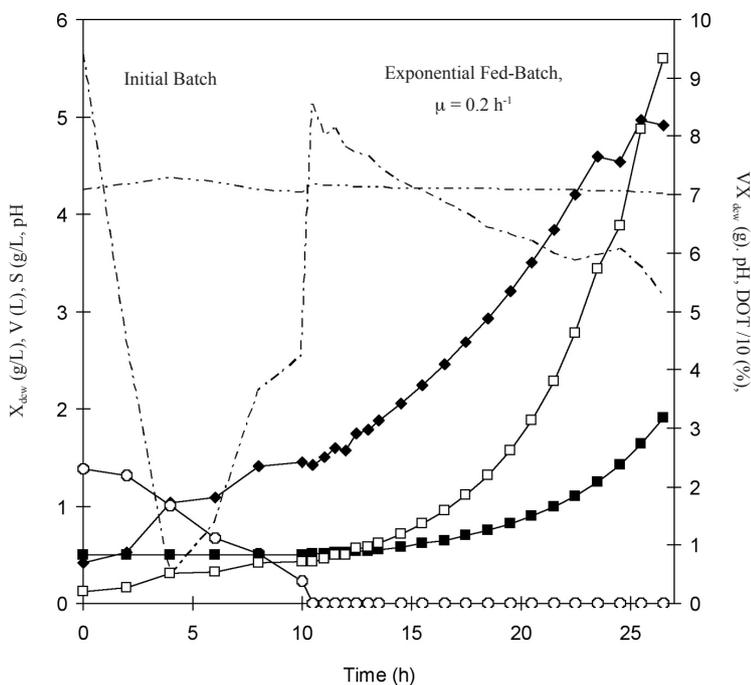
Fig. 2: The time course of exponential fed-batch fermentation at  $\mu = 0.2 \text{ h}^{-1}$  using glycerol as the carbon source in a 2 l fermenter. Symbols represent (◆)  $X$ ; (○)  $S$ ; (■)  $V$ ; (□)  $VX$ ; (---) pH; (—) % DOT/10. Arrow indicates the start of feeding for the fed-batch fermentation
