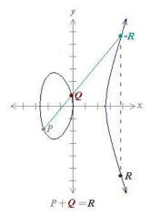
Figure 1: Elliptic Curve Addition
