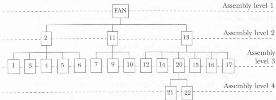
Fig. 5: Components assembly level
