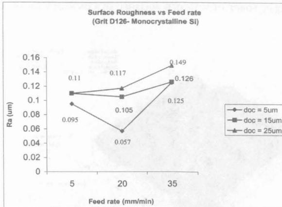
Fig. 5: Surface roughness obtained when silicon dies were precision ground at different levels of depth of cut and feeds
