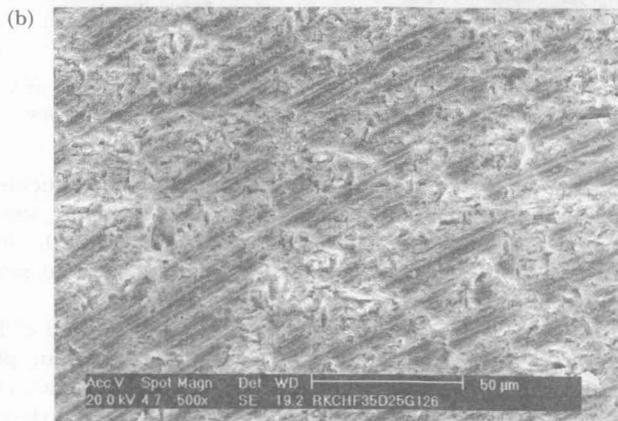
Fig. 6: SEM pictures of ground Si. The surfaces consist of (a) microfractures and (b) grinding streaks
