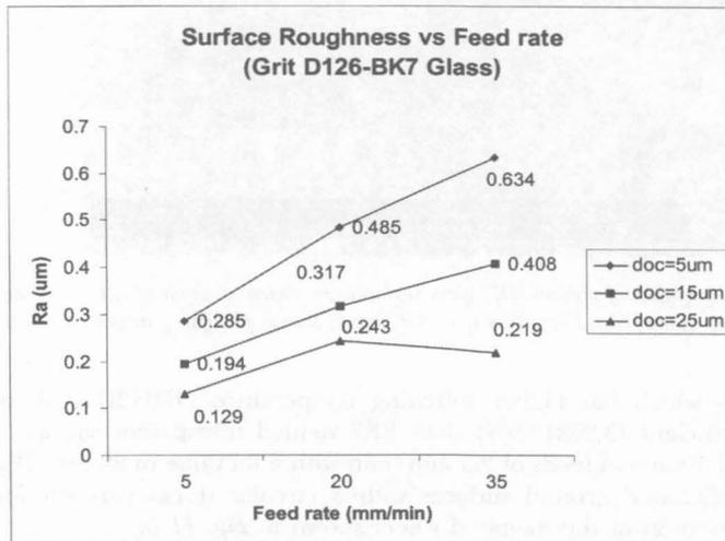
Fig. 9: Surface roughness obtained by plano grinding at different feeds and depth of cuts on BK7 glass
