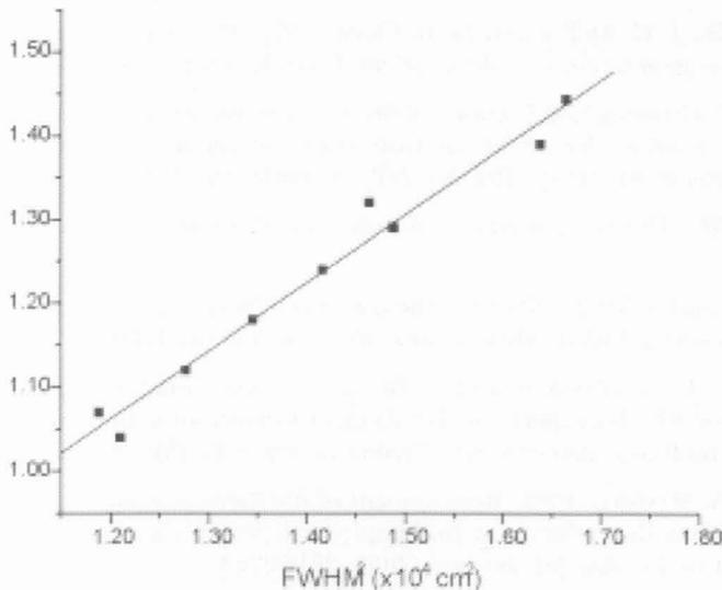
Fig. 6: Liquid mixture thermal diffusivity versus  $(\text{FWHM})^2$
