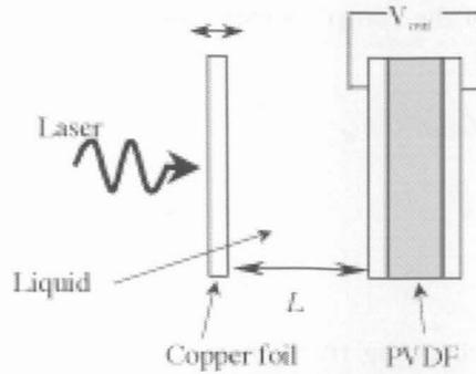
Fig. 1: Schematic diagram of thermak-wave resonant cavity cell
