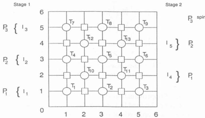
Fig 2. The solution domain  $\Omega^h$  with the horizontal zebra line (HZL) ordering strategy for o type of points
