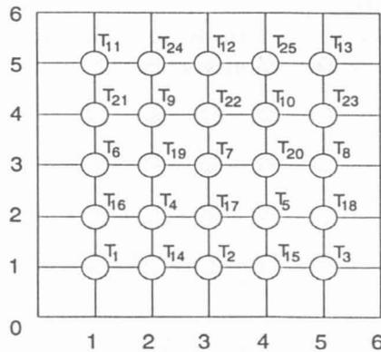
Fig 1. The solution domain  $\Omega^h$  with the chessboard (CB) ordering strategy for o type of points
