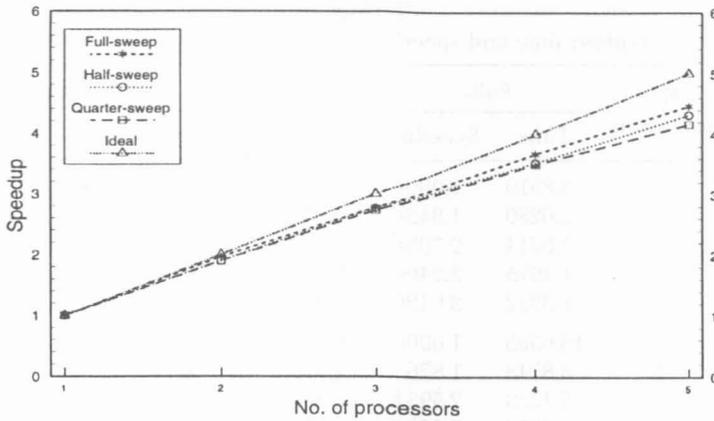
Fig 5. Speedup versus number of processors for  $n=100$
