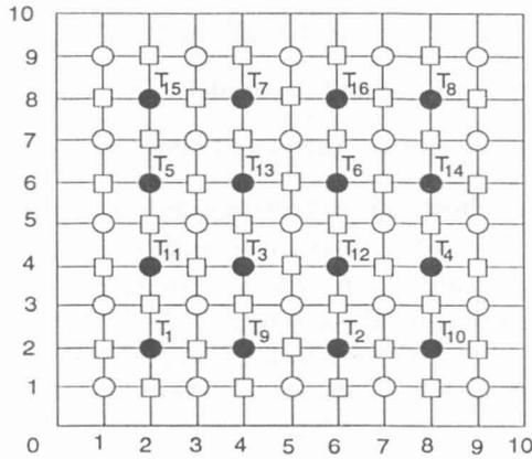
Fig 3. The solution domain  $\Omega^h$  with the CB ordering strategy for ● type of points
