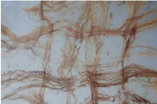
Figure 3: Biocomposite materials developed from kenaf fibers
