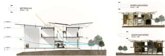
Figure 8: The raised floor and spaces between the double-bamboo structures allow natural ventilation and daylight to infiltrate across the whole scheme.
