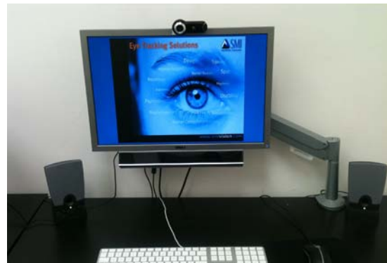
Figure 1: Desktop based eye-tracking equipment where Shuttle-1 was used by researchers to monitor eye-tracking experiment and Shuttle 2 was equipped with an eye-tracking infrared sensor to track the participants eye movements.
