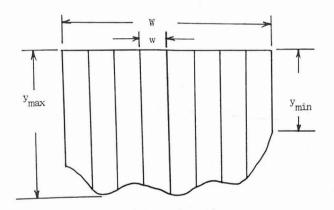
Fig. 2. Depth of infiltrated water along a section across the furrow field
