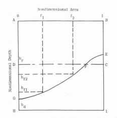
Fig. 3. Averaged water distribution profile over an irrigated furrow field
