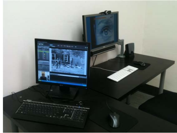
Figure 2: Eye tracking equipment in the Perception and Usability Testing Laboratory at Virginia Tech, Blacksburg, Virginia. An operator controls the foreground computer, and a participant sits in front of the screen in the back
