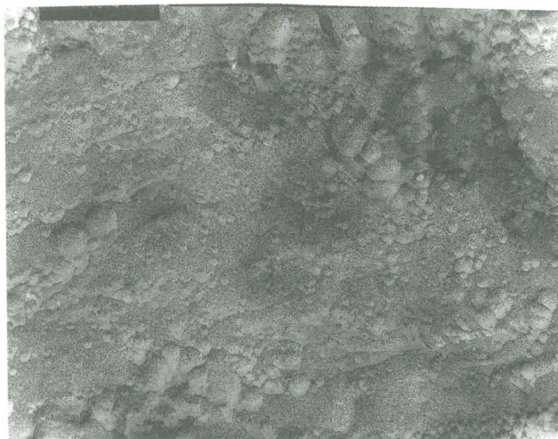
Plate 1. Freeze-fracture electron micrograph of an aerosol-OT water-in-heptane microemulsion containing polyethylene oxide (mol. wt. = 105,000) at 55,000 magnification. Note the relatively small number of large droplets compared to a larger number of smaller droplets in the background
