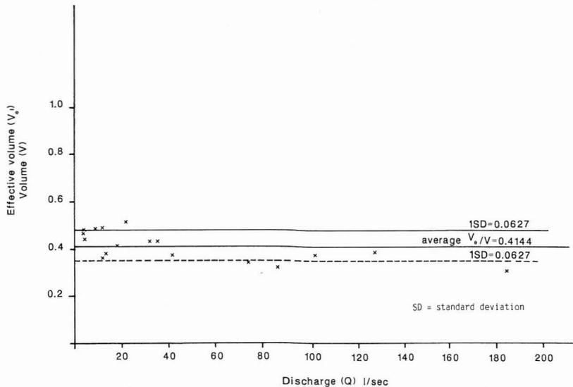
Fig. 4. Immobile fraction as a function of discharge for Crimble Beck
