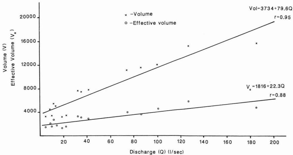
*Fig. 3. Reach volume and ADZ volume as functions of discharge for Crimple Beck*
