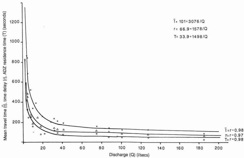
Fig. 2. Mean travel time, time delay and ADZ residence time as functions of discharge for Crimple Beck
