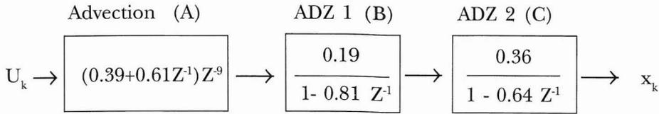
where block A represents the advective effects (pure-time delay of 9 sampling periods) and the value  $0.39 + 0.61 Z^{-1}$  is to allow for the additional “non-integral” time delay which gives rise to the requirements for the 2 “b” parameters. Blocks B and C represent 2 unequal ADZ elements in series.
