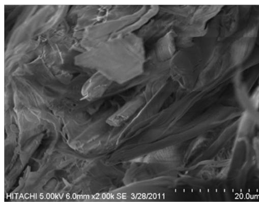
Fig.3: Tensile specimen at 100kGy without cross linking
