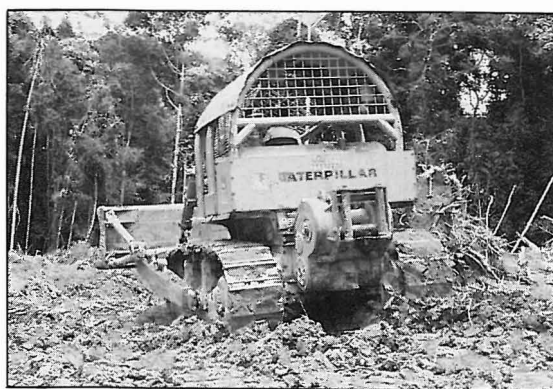
Plate 2: The track-type tractor used for vehicular compaction test
