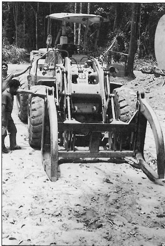
Plate 1: The rubber-tyred grapple loader used for vehicular compaction test
