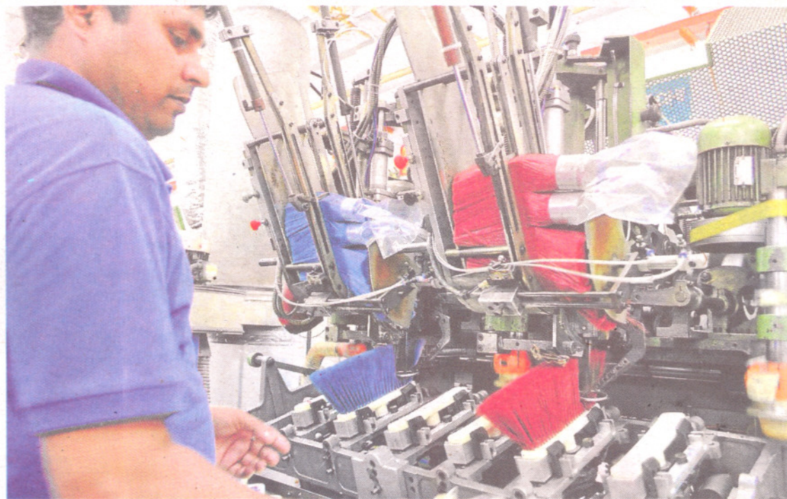
Adding colour: Coloured nylon bundles await a permanent fix to their heads at the factory. Like fashion, brooms are also subject to colour trends.
