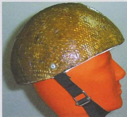
Fig 1. The helmet with bio-composite shell
