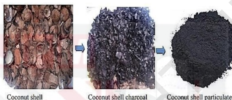
Figure 2.6 : Production process products: coconut shell – coconut shell particulate (Source: Oluwole et al., 2017)
