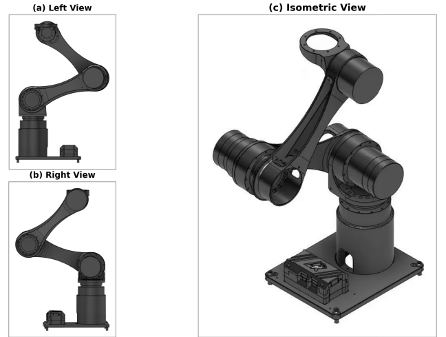
FIGURE 16. Computer-aided design (CAD) views of the 4-DOF manipulator: (a) left, (b) right, (c) isometric. Reach \approx 538 mm.
