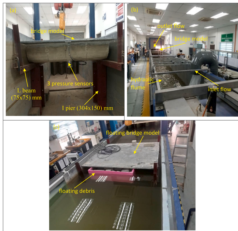
Fig. 2. Experimental setup of the floating bridge model: (a) model installation, (b) bridge submersion, and (c) flow and debris loading acting on the bridge.
