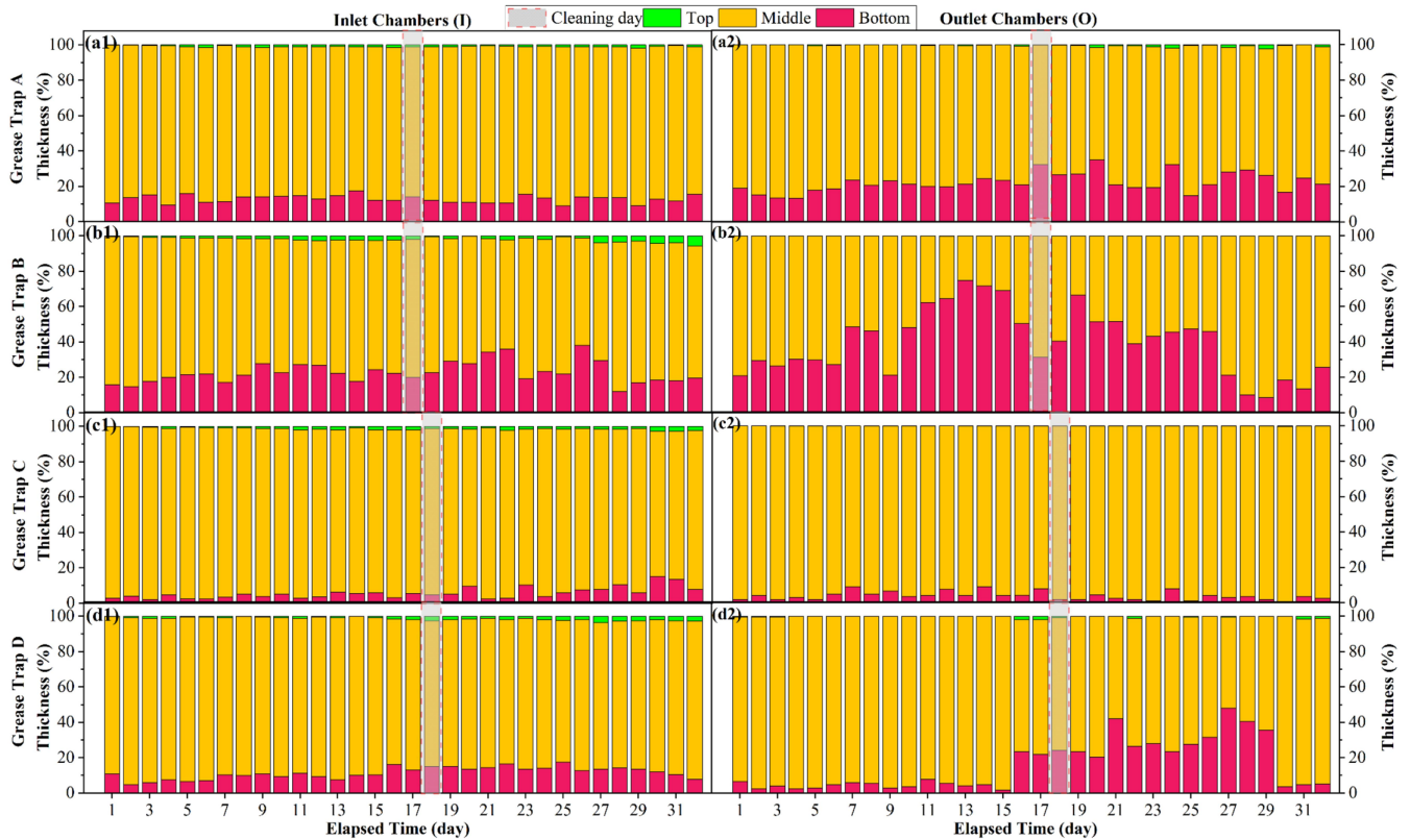
FIGURE 2 | Normalized three-layer thickness profiles (%) of Grease Traps A–D over a 32-day site investigation. Subplots (a1–d1) represent the inlet chambers (I), while subplots (a2–d2) represent the outlet chambers (O). Vertical markers on Day 17 (Grease Traps A and B) and Day 18 (Grease Traps C and D) indicate desludging and cleaning events.
