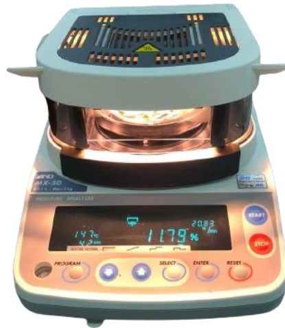
Figure 3.11: Leaf Moisture Content Measured using Moisture Analyzer
