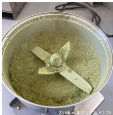
Figure 5 : Preparation of Grass Meal (Grinding)
