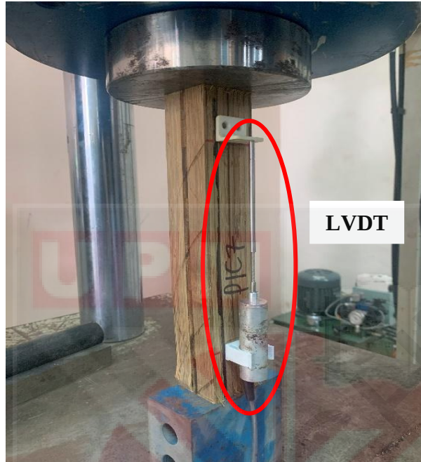
Figure 5.8: Compression Parallel to the Grain Test Set-up
