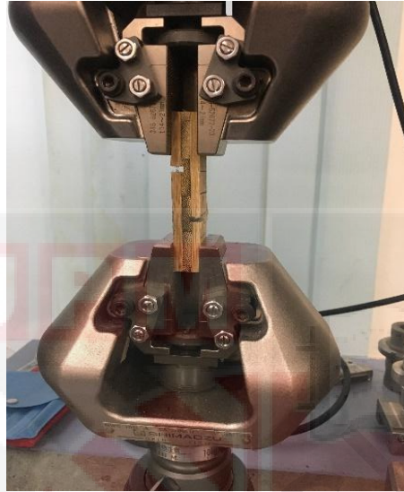
Figure 4.6: Specimen Tested using UTM Shimadzu Machine
