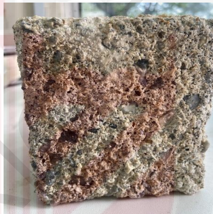
Figure 4.10: Concrete for acid resistance test at 28 th days (a) COM1 (0% aluminum dross) (b) COM2-S3 (5% aluminum dross sample 3) (c) COM3-S3 (10% aluminum dross sample 3) (d) COM4-S3 (15% aluminum dross sample 3)
