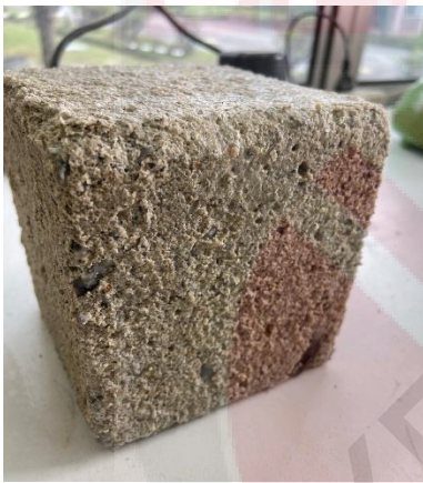
Figure 4.10: Concrete for acid resistance test at 28 th days (a) COM1 (0% aluminum dross) (b) COM2-S3 (5% aluminum dross sample 3) (c) COM3-S3 (10% aluminum dross sample 3) (d) COM4-S3 (15% aluminum dross sample 3)
