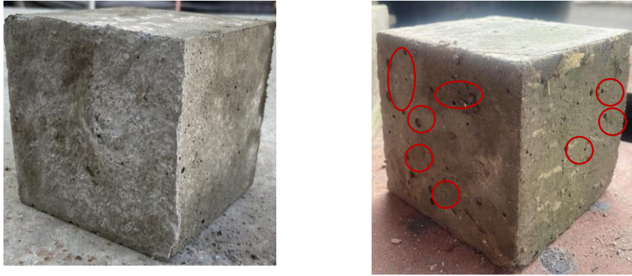
Figure 4.4: (a) Concrete mix COM1 (0% aluminum dross), (b) Concrete mix COM2 (5% aluminum dross), (c) Concrete mix COM3 (10% aluminum dross), (d) Concrete mix COM 4 (15% aluminum dross)
