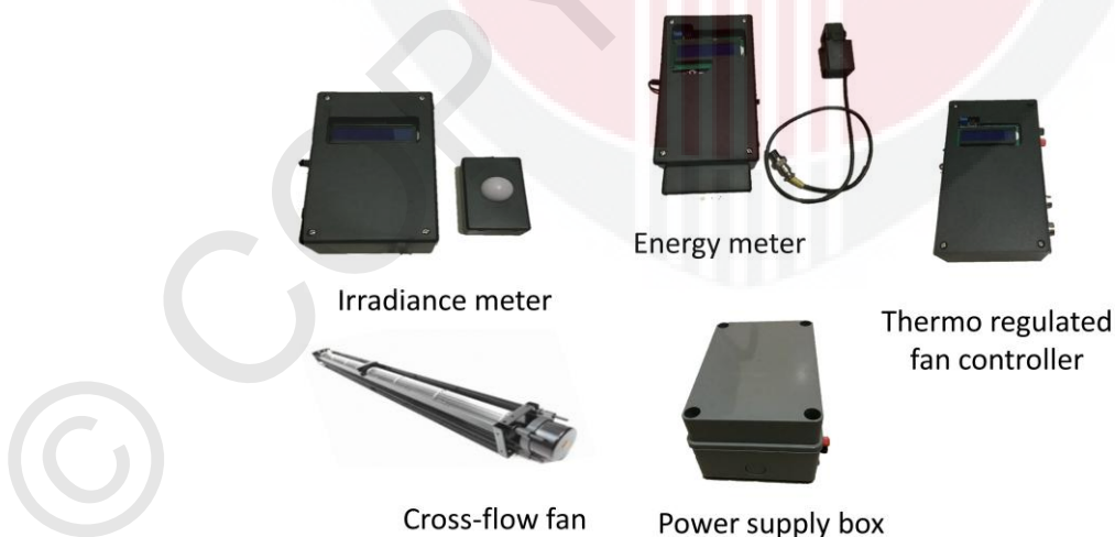
Figure 4.1: Meter and devices used in the thermoregulated air-cooling retrofitted PV system experiment
