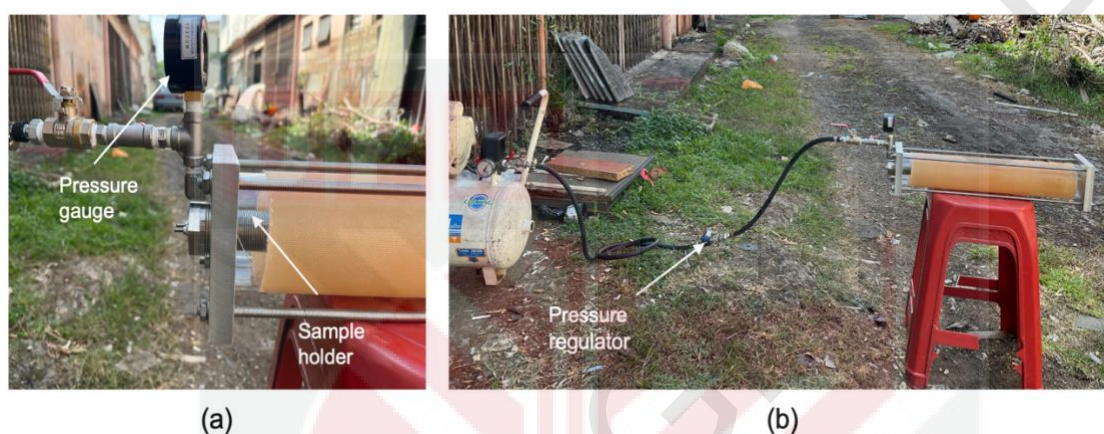
Figure 3.15: Crawford type strand burner setup (a) close-up view on the pressure gauge and sample holder setting and (b) full view
