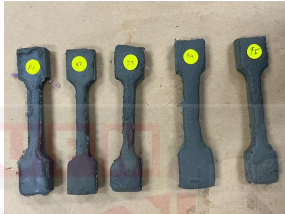
Figure 3.13: Propellant dog bone sample according to JANNAF standard specimens
