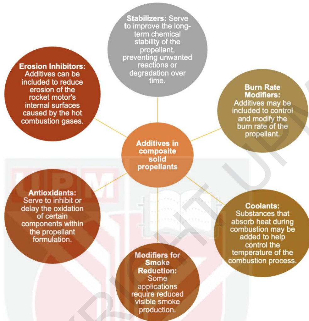
Figure 2.5: Common types of additives used in composite solid propellant rockets
