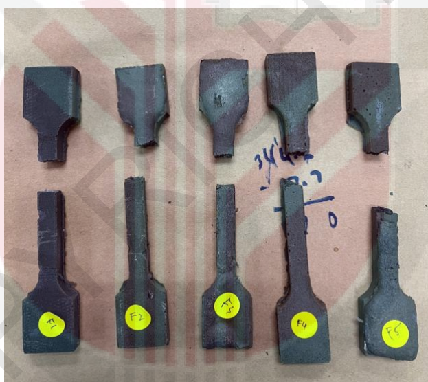
Figure 4.20: Physical state of dog bone samples after uniaxial tensile test
