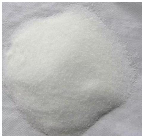
Figure 2.6: Ammonium perchlorate (AP) as a white, odourless crystal (Source: Yeh et al., 2021)
