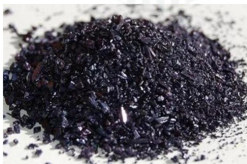
Figure 2.9: Physical structure of potassium permanganate ( \text{KMnO}_4 ) (Source: Wu et al., 2019)
