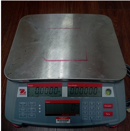
Figure B.9: OHAUS Ranger Count 4000 Weighing Scale for Precise Mass Loss Rate Measurement
