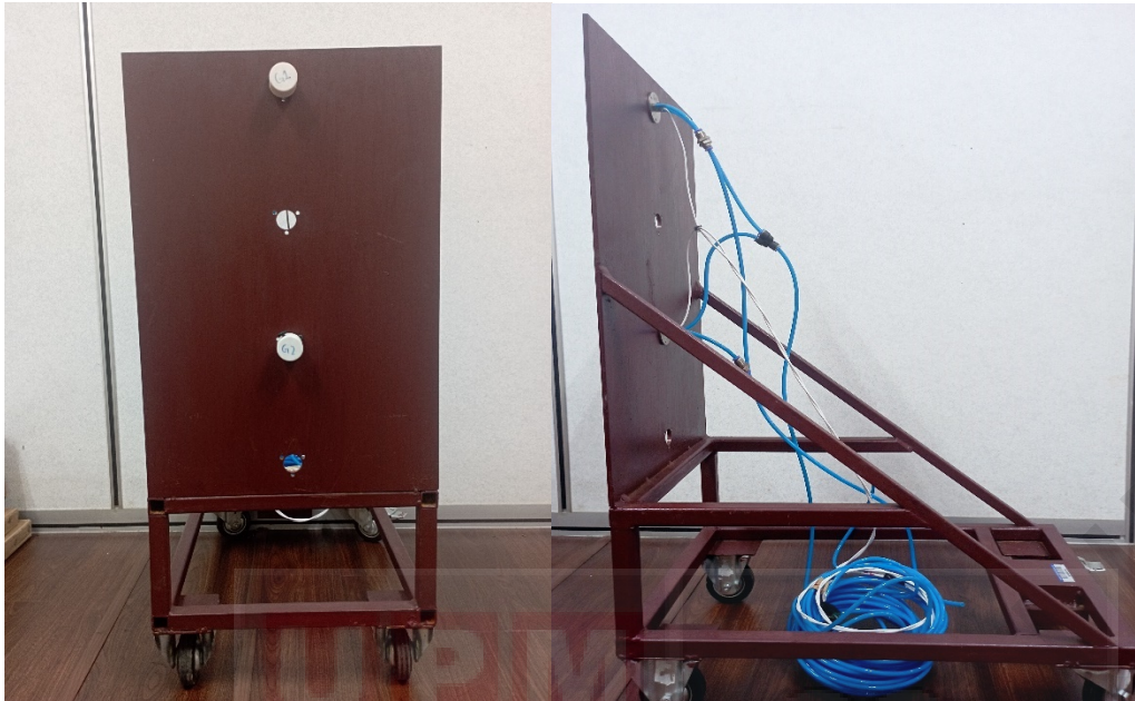
Figure B.3: Heat Flux Gauges Mounted on a Mobile Trolley for Heat Flux Measurements
