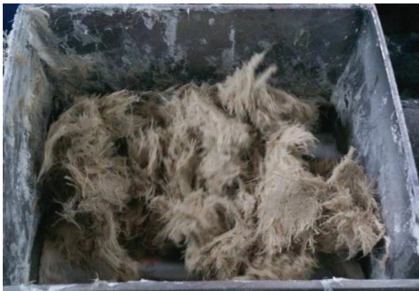
FIGURE 3 | Mixing kenaf-reinforced BMC.
