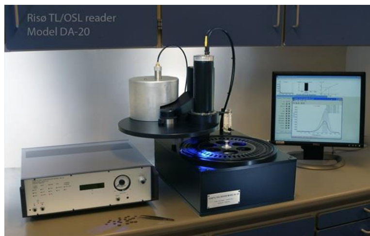
Figure 3.64: Risø TL/OSL reader equipped with beta irradiator (Nielsen, 2023)
