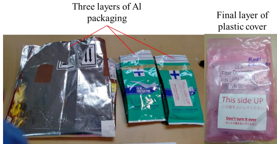
Figure 3.73: Packaging used to protect FM from external radiation
