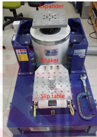
Figure 3.45: AT random vibration test setup with an expander attached to the armature of the shaker
