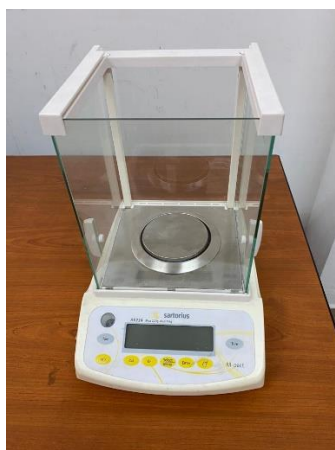
Appendix B9. A High-accuracy weighing scale (Sartorius, M-pact AX224)
