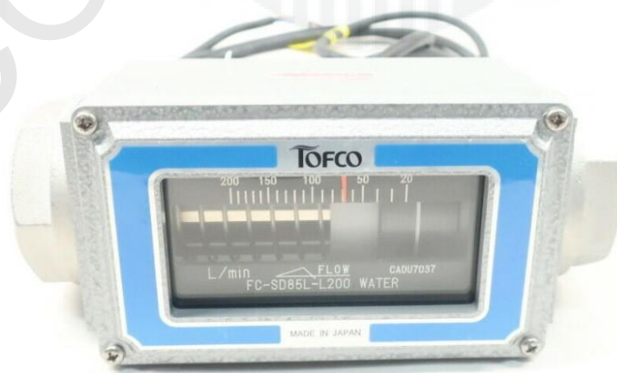
Appendix B8. A flow meter (FC-SD85L-L200)
