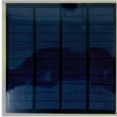
Figure 4.1: Damaged M1 sample (30kV)
