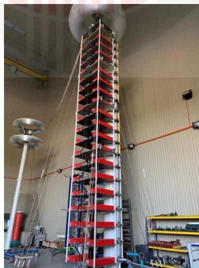
Figure 3.4: The multistage Marx impulse generator
