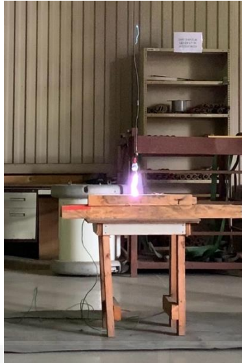
Figure 3.7: Lightning strike induced on sample
