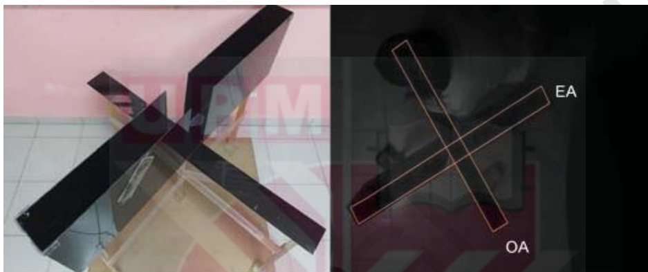
Figure 4.3 : Experimental setup during modified elevated plus maze test (mEPM). The device plus (+) shaped with two enclosed arms (EA) and two open arms (OA). All the arms linked by central square
