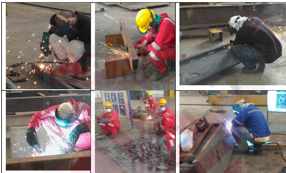
Figure 2.3: Ergonomic position of a welder performing welding activities at the container framework fabrication area
