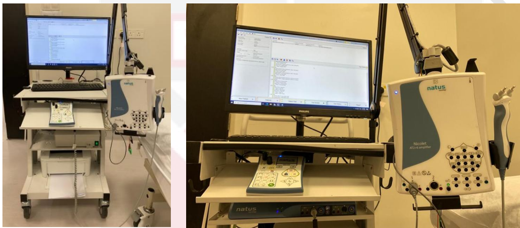
Figure 3.1: Natus Nicolet AT2 Amplifier (Natus Neurology, USA) equipment used to conduct EMG examination.
