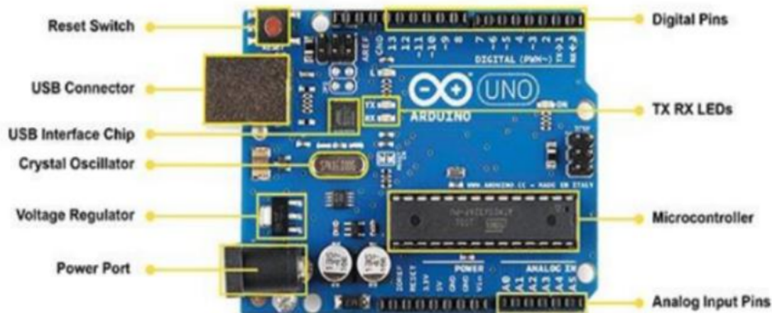
Figure 2. Components of Arduino UNO board
