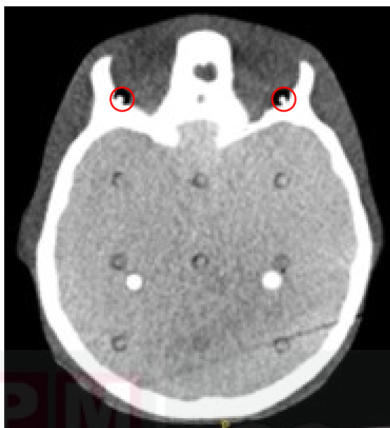
Figure 4.38: Placement of TLD-100 chips (red circles) within the eye dosimetry holes for eye organ dose measurement
