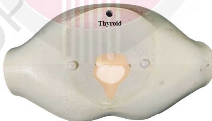
Figure 3.24: Thyroid dosimetry hole filled with soft tissue plug on the 8 th slice of ATOM® dosimetry phantom
