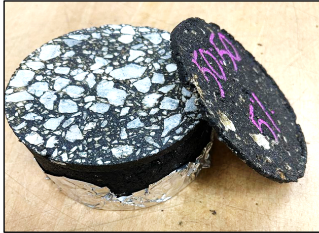
Figure 3.16: Trimmed Marshall specimen for dynamic creep test
