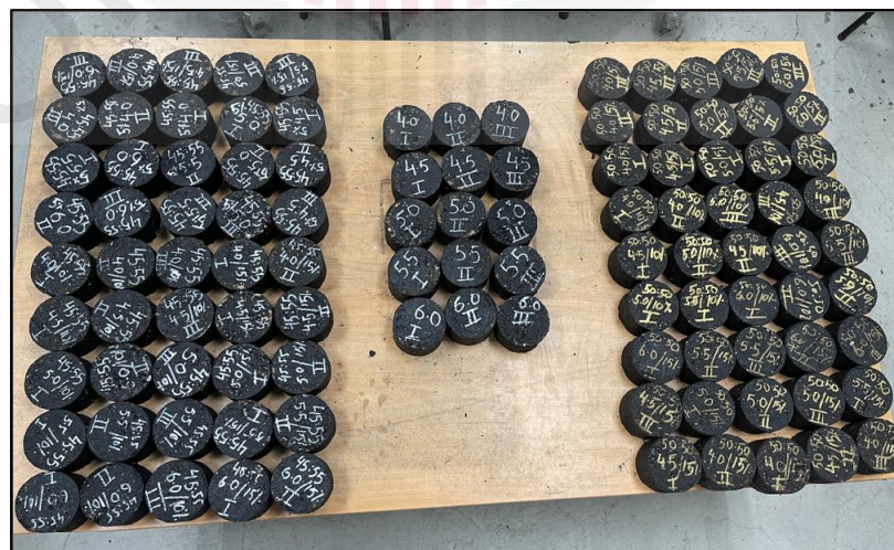
Figure 3.13: Cylindrical compacted specimens
