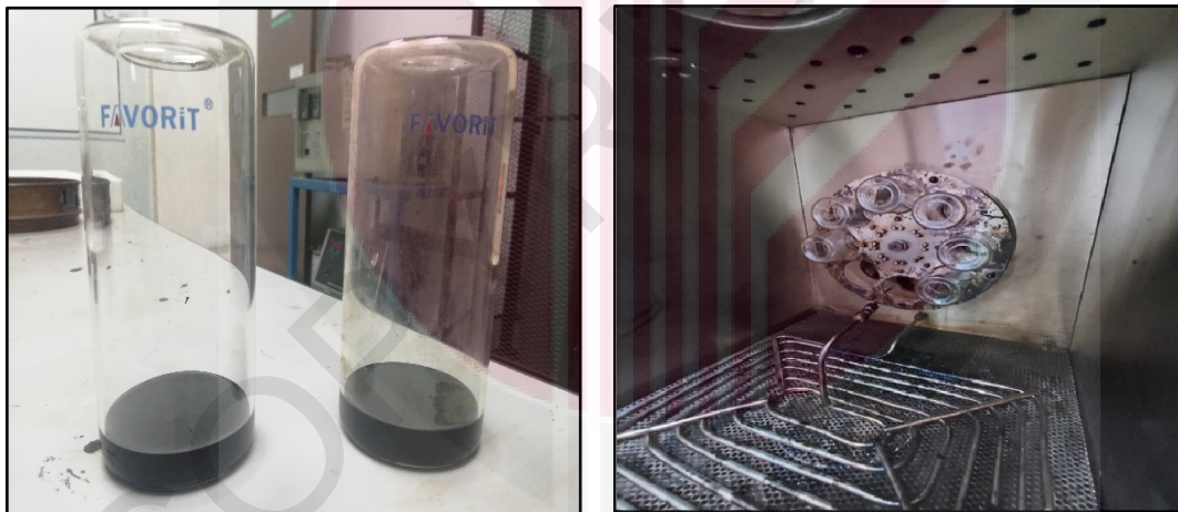
Figure 3.6: Short-term ageing of base and modified bitumen using RTFO
