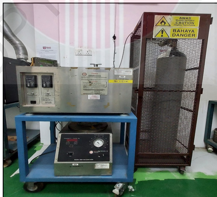
Figure 3.7: PAV and vacuum chamber for bitumen long-term ageing
