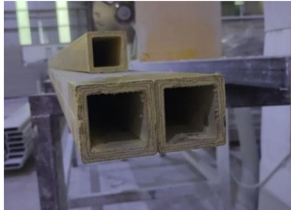
Figure 3.16: Kenaf/glass reinforced hybrid square hollow pultruded profiles
