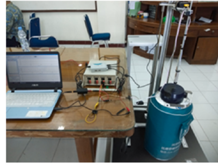
Fig. 2. (a) Schematic of the sample sketch, perspective view, and Cu/Ni sample, and (b) Low-temperature measurement research apparatus.
