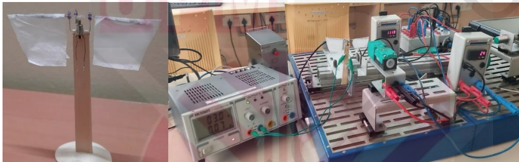
Figure 3.27 : SC-SDL Design III with Flapping Frequency Measuring Setup
