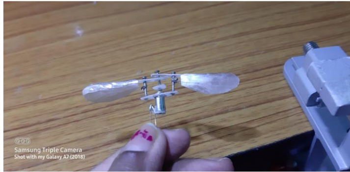
Figure 3.28 : Mosquito Wing Shaped Plastic Wing Attached to the Handmade SC-SDL Mechanism Design
