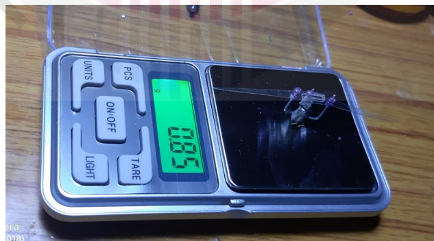
Figure 3.25 : Weight of Compact Handmade SC-SDL Design Mechanism with Motor (without Wings)
