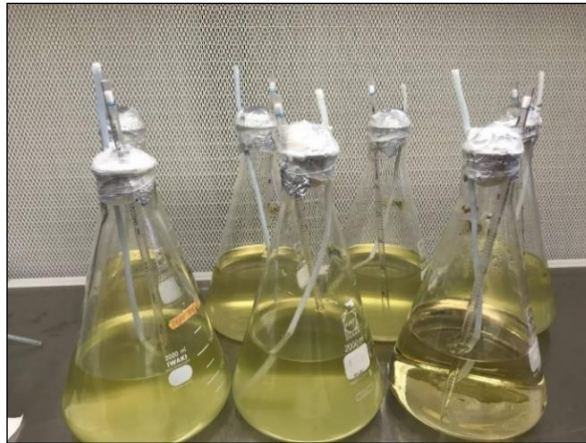
Figure 3.3 : An Erlenmeyer Flask Containing Aquaculture Wastewater at Day 0 Bioremediation Process
