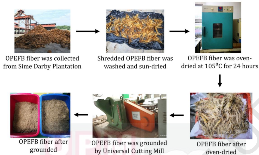
Figure 3.7: Flow diagram for biomass preparation
