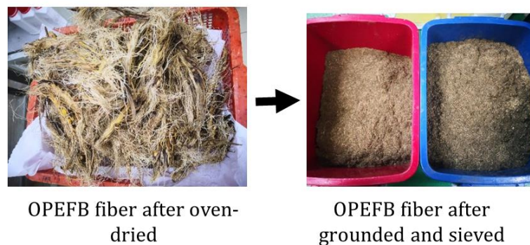
Figure 4.29: OPEFB sample after dried, ground and sieved
