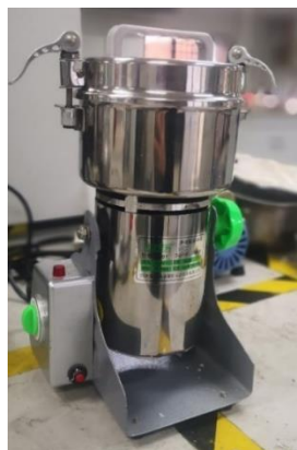
Figure 3.10: Grinder used to grind the cellulose after the treatments
