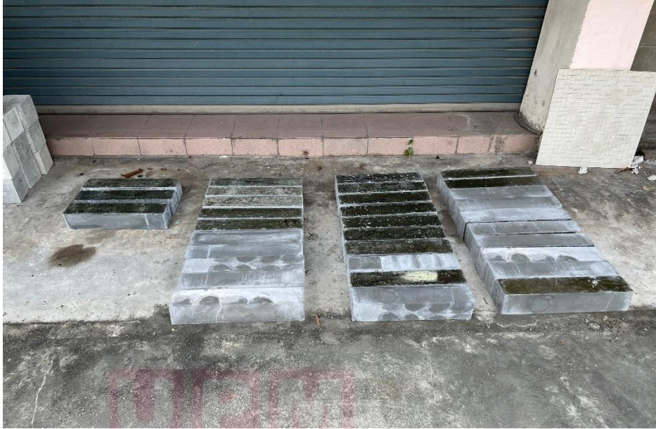
Figure 3.13 : Prism samples of 100×100×500 mm
