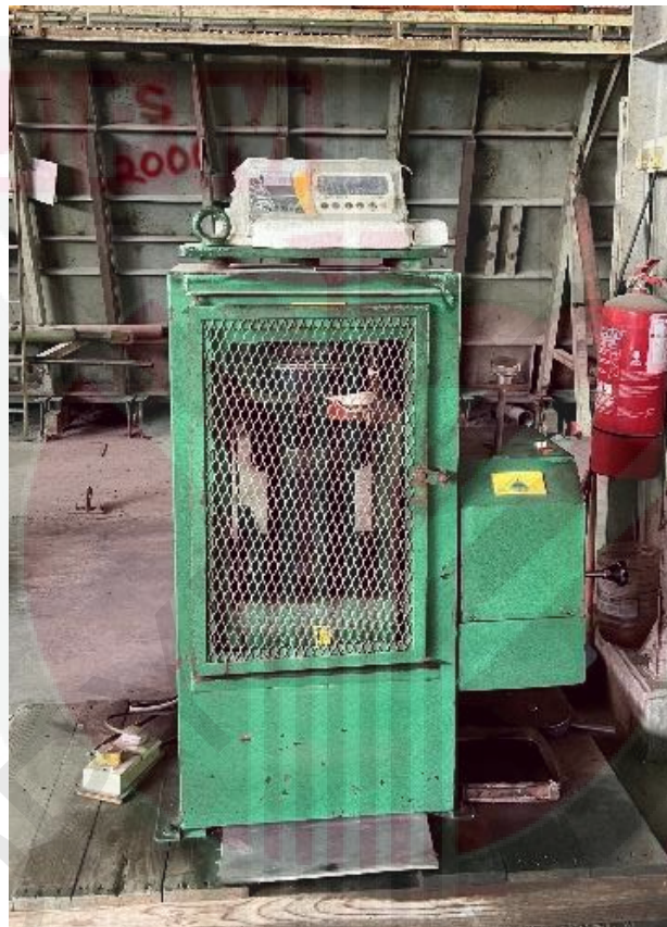
Figure 3.17 : Hydraulic compressive machine with maximum compressive force of 2500 kN
