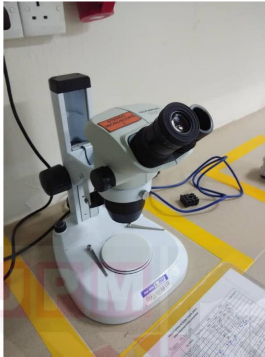
Figure 3.23 : Photo of stereomicroscope for pore analysis of sample
