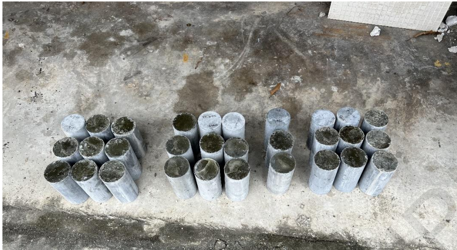
Figure 3.16 : Cylindrical samples of 100 mm (diameter) × 200 mm (height)
