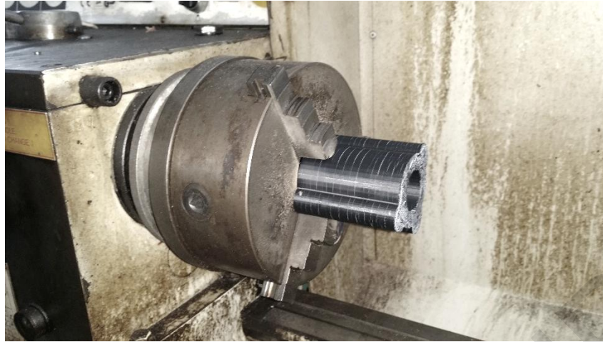
Figure 3.15: Swirl IM prototype device finishing process using the ZMM SLIVEN CU 400M universal lathe machine.
