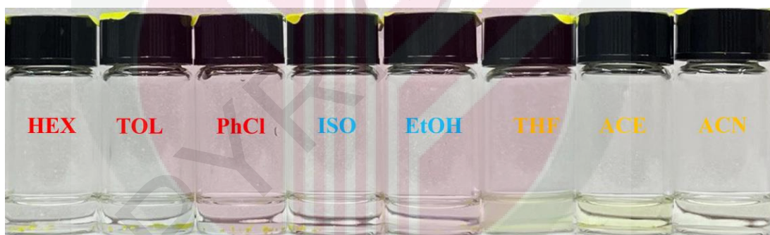
Figure 4.3: MBB crystal powder with different types of solvent; Hexane (HEX), toluene (TOL), chlorobenzene (PhCl), 2-propanol (ISO), ethanol (EtOH), tetrahydrofuran (THF), acetone (ACE), and acetonitrile (ACN) (word in red: non-polar; word in blue: polar protic; word in yellow: polar- aprotic).
