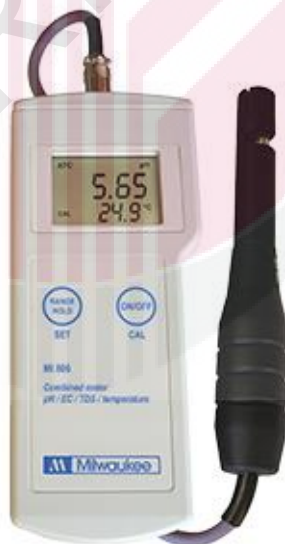
Figure 3.3: A pH meter used for pH measurement
