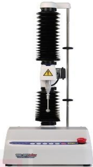
Figure 3.8: A texture analyser used for Texture Profile Analysis
