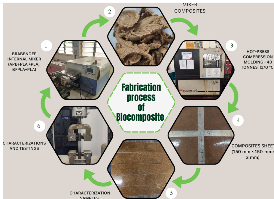
Fig. 5. Fabrication of plant ash bamboo reinforced PLA composites.
