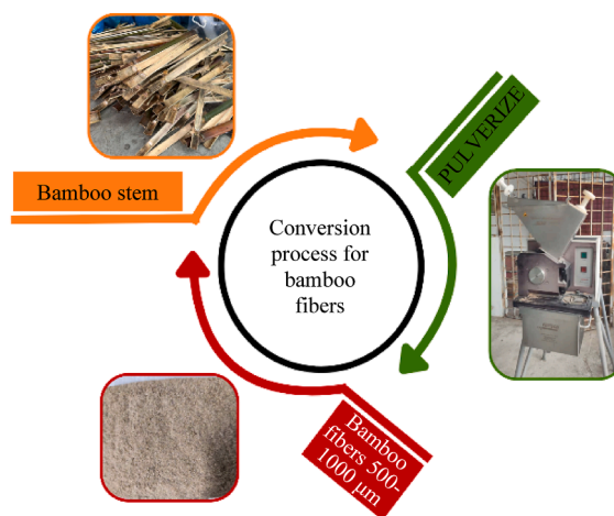
Fig. 3. Process of making bamboo fibers.
